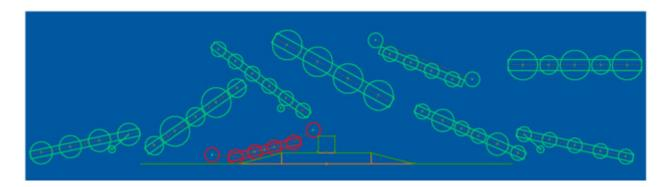
Each rail shows a few of the many conceptual ideas that we went through. The one in red represents what decision we made. The drive rail would have 4 inch wheels on a large drop center of 1 inch. The wheels would be 2 inches wide so we did not lodge the wheels in between the blocks in the Rough Terrain. Most of our time was spent deciding what the configuration would be. Once we knew that, power transmission was easy.
