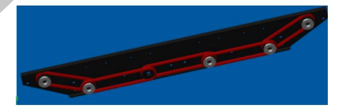
The gearbox feeds into the boxtube and chain runs through the boxtube as seen previously. Assembly for this design can be a bit tricky, however, the chain rarely needs to be serviced if done correctly due to the shielding.
